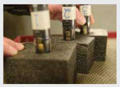
Temperature gauges being prepped for test
