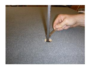
Using the 10mm wrench, lower the spare tire from the bottom of the vehicle.
