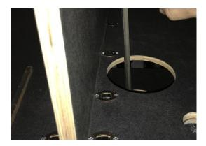
Insert the spare access rod through the hole in the top of the Vault and into the spare tire release. You may have to rotate the tool to line it up with the release.
