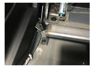
Move the bracket back into place lining up the holes in the brackets with the factory bolts and Plus-Nuts. Bolt down the bracket using the factory bolts in the back.
