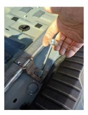
Bolt down the front of the bracket using two  $5/16 \times 1$  1/2" hex bolts &  $1 \cdot 1/4$ " washers on the outside feet and the supplied  $5/16 \times 5$ " bolts and washers on the middle two feet.
