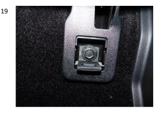
Remove the bolt using a 18mm socket. Install the tie down strap brackets & re-attach the factory bolt.
