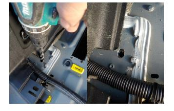
Using a 1/2" drill bit, drill out the foam in the side holes on both sides of the vehicle for plus nut installation.
