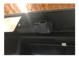
Attach the antenna sensor to the bottom of the cargo cover with the supplied 10-24 x 1/2" machine screws.
