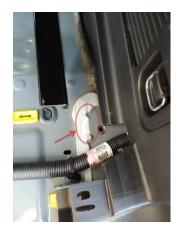
Note: Some of the rubber sealant may have to be trimmed down to allow the bracket feet to sit flat.
