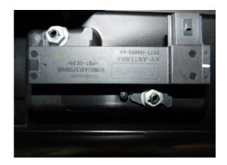
Remove the antenna sensor from the under side of the cargo tray using a 10mm socket.
