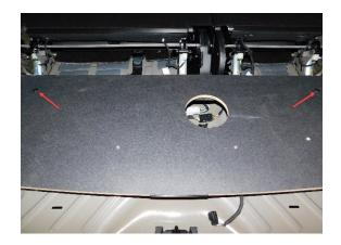
Place cargo cover onto the bracket ensuring the holes are aligned. Secure rear of cargo cover to the bracket using (2) 5/16-18 connector bolts.
