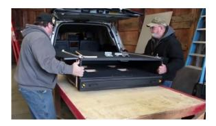
Fold down the 3rd row seat. With help, carefully install the TruckVault into the cargo area.
