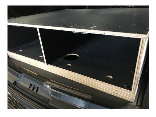
Using (3) 5/16" x 3" hex bolts and fender washers, line up the bolts with the inserts in the front of the cover.
