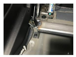
Place the mounting bracket in the rear of vehicle, aligning back holes in the bracket to the holes in the floor of the vehicle, and secure using the bolts factory bolts. Leave bolts loose as you will need to remove the bracket for plus nut installation.
