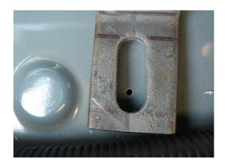
Carefully check underneath the vehicle to make sure there is nothing below the bracket front holes such as wiring, gas tank, spare tire etc. Drill a 1/8" pilot hole through the front of the bracket hole. (Note: A minimum 5" long drill bit must be used to go through upper and lower layers of the cargo area.) Move the mounting bracket out of the way. Drill a 3/8" hole where the 1/8" pilot hole was drilled.
