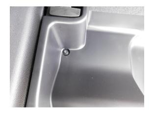
Open the cargo cover lid and remove the jack storage compartment using the 10mm socket. You will need to relocate the jack and accessories.
