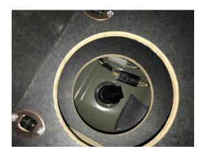
Reach in through the bottom of the TruckVault and through the cargo cover. Remove the cover cap from the spare tire access hole.
